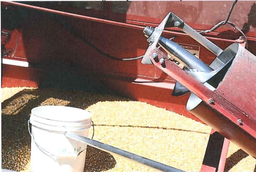
Fig. 1. Sampling corn for aflatoxin analysis in the experiments. The bucket is held under the auger as the combine moves through the plot so that only 11-18 lb. of a plot is sampled.
